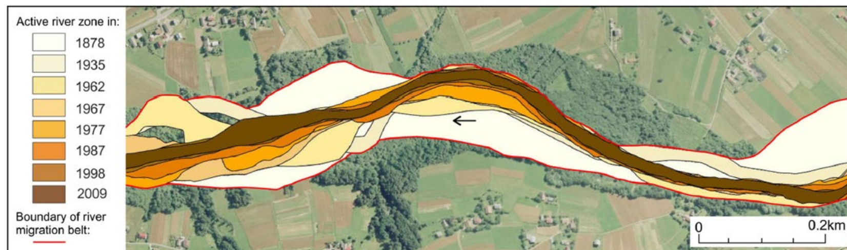
Fig. 3. Extent of the active zone of the Biała River digitized on the archival maps and orthophotos from the period 1878–2009 and the belt of river migration in this period shown for a fragment of the mountain section of the planned erodible corridor.
